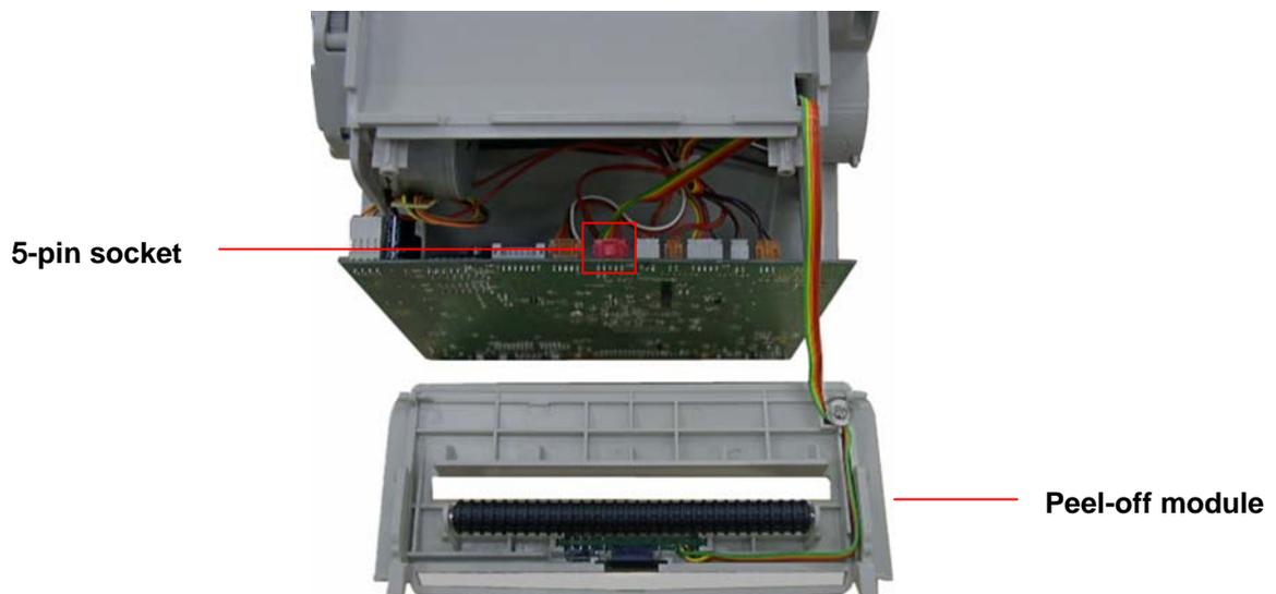
4. Embed the tenons into the both sides mortise of lower inner cover and close the peel-off cover.
