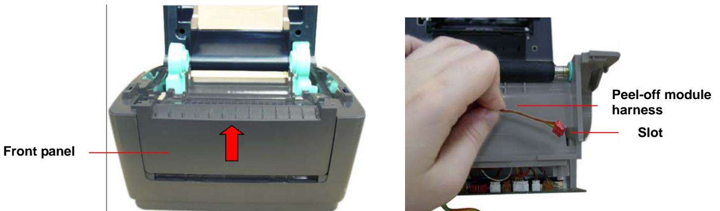
3. Plug in the peel-off module harness connector to the 5-pin red socket on the main board.
